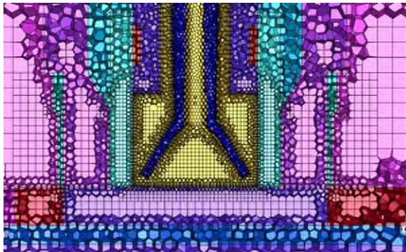
Picture 1: Computational grid for thermal simulation with a magnified representation of the NanoCube exposure device. The aerosol sections are in yellow, the other sections are either components or air sections.
