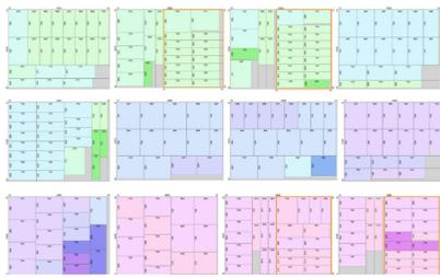
AutoPanelSizer computes this cutting layout in 0.3 seconds. It has been taken into account that only 3 destacking stations are available. Parts with the same color must be destacked together.
