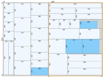
Cutting layout with head cut: The cutting plan is divided into the "head plan" (on the left) and the "main plan" (framed in orange). Both contain three cutting stages. The strips on the main plan are rotated by 90 degrees.
